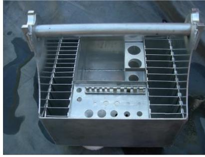
There are other possible tool organizing modules that keep your tools in place. The first tote box I made in 1982 was made of a nice piece of wood with aluminum sides. I dovetailed the joints and installed the handle in a similar fashion to the specially machined Cliffhanger attachment block used today. I glued two-two by fours laid on their sides together. I drilled the appropriate holes in the wood to hold my tools in place. This method could be used in the Cliffhanger aluminum tote box.
